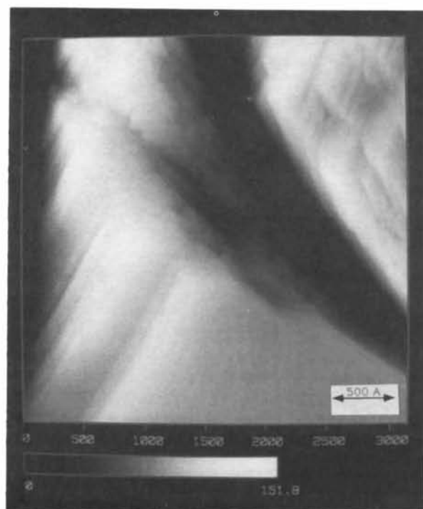
Fig. 5. STM image of a 300 Å Pt thin film of the sample in Fig. 4 after being annealed in \text{H}_2 at 1273 K for another 3 h. The Z axis, in ångströms, is shown by the gray-scale insert at the bottom of the figure.
